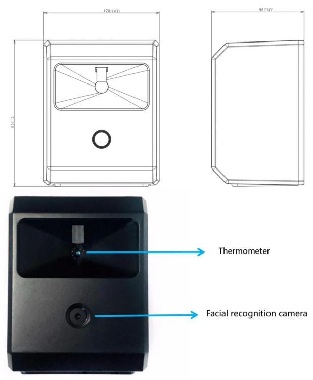
The terminal includes the CPU and AI algorithms. You can see the interface overview below.
