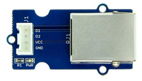
The Grove-RJ45 Adapter is a module which can convert a standard Grove connector to a RJ45 connector. Universal 4-Pin Grove cables can not meet the requirements when Arduino remote connect and control Grove module. Through two RJ45 adapter and a cable, It is able to achieve communication between Arduino and Grove module. This help solve the problem that Arduino and Grove are not convenient to connect because of the distance issue.
