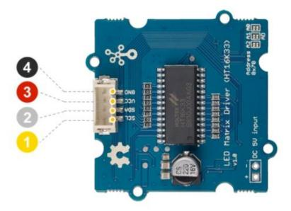
4 GND: connect this module to the system GND
