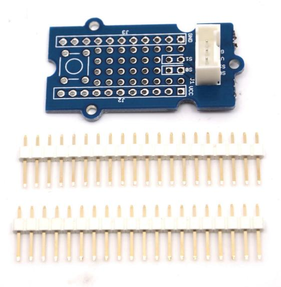
This Grove allows you to add your own circuitry or components to your Grove system prototypes. It gives you access to all four lines from the grove connector cable – S0, S1, VCC and GND. There is also a reserved space for a normally-open button. Standard 2.54mm spacing makes it easy to install normal DIP-format ICs and other components onto the board.
