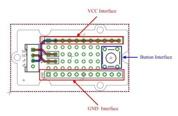
VCC and GND of the Grove interface are routed out as two buses as shown above. You can find soldering pads of Sig0 and Sig1 between two power buses.
