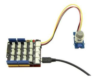
Connect the Grove - Gas Sensor(MQ5) to A0 port as shown in the picture above.
