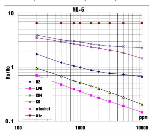
According to the figure, we can see that the minimum concentration we can test is 200ppm and the maximum is 10000ppm, in a other word, we can get a concentration of gas between 0.02% and 1%. However, we can't provide a formula because the relation between ratio and concentration is nonlinear.
