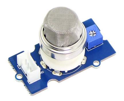
The Grove - Gas Sensor(MQ5) module is useful for gas leakage detection (in home and industry). It is suitable for detecting H2, LPG, CH4, CO, Alcohol. Due to its high sensitivity and fast response time, measurements can be taken as soon as possible. The sensitivity of the sensor can be adjusted by using the potentiometer.
