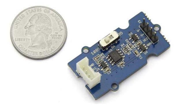
This Grove is designed for precise differential-input amplification. Input the differential signals of your sensor to this module through the male pins, then your Arduino will get a precisely amplified output from the Grove interface. The gain scale factor is selectable. You can get a 35 times or 1085 times amplification via a switch on the board.
