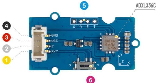
**④ GND:** connect this module to the system GND
