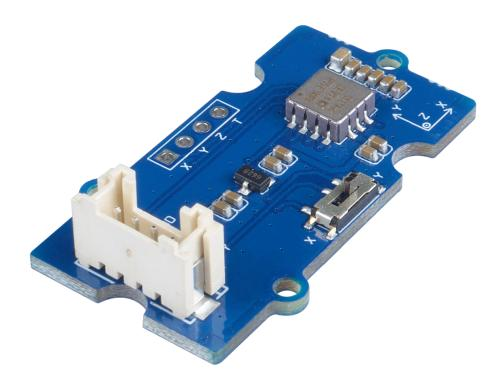
**Grove - 3-Axis Analog Accelerometer ±20g (ADXL356B)**
