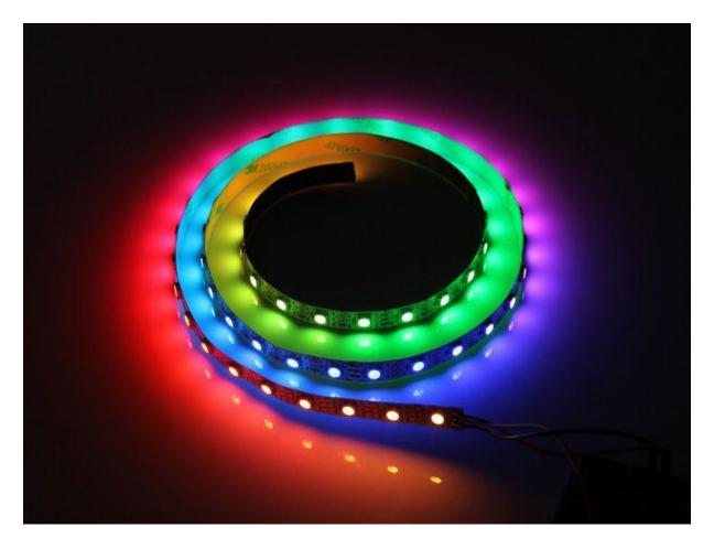
Digital RGB LED Flexi-Strip is an intelligent light source consist s of WS2812B RGB LED with Integrated Driver Chip. The control circuit and RGB chip are integrated in a package of 5050 components.
