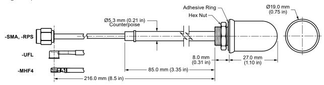
Figure 1. ANT-W63-WRT-ccc Antenna Dimensions
