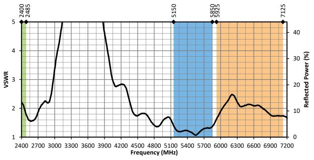
Figure 3. ANT-W63-WRT-ccc VSWR with Frequency Band Highlights
