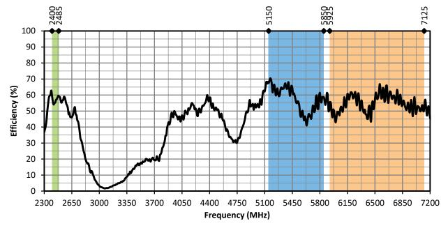
Figure 8. W63WS1 Series Antenna Radiation Efficiency, Straight
