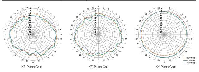
Figure 9. ANT-W63WS1 Antenna Radiation Patterns, Straight
