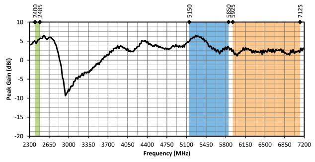
Figure 13. W63WS1 Antenna Peak Gain, Edge-Bent
