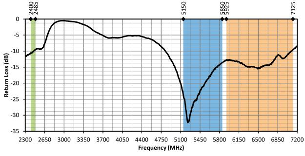
Figure 12. W63WS1 Antenna Return Loss, Edge-Bent
