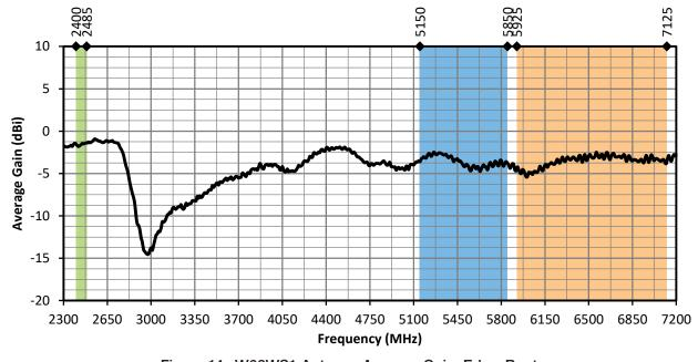
Figure 14. W63WS1 Antenna Average Gain, Edge-Bent
