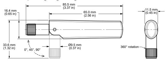
Figure 1. ANT-W63WS1 Antenna Product Dimensions
