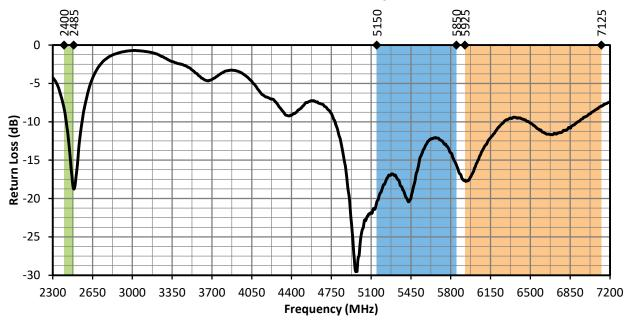
Figure 5. W63WS1 Return Loss, Straight
