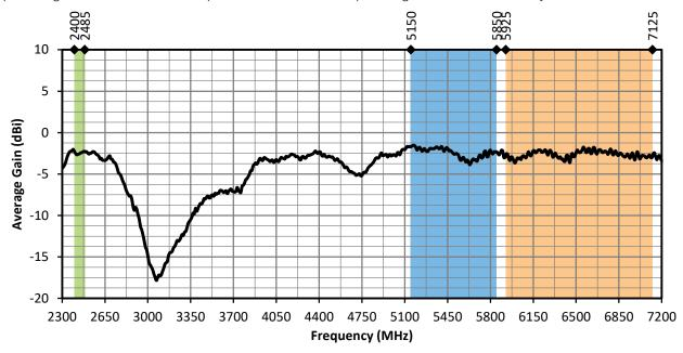
Figure 7. W63WS1 Antenna Average Gain, Straight
