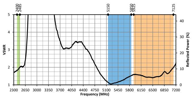
Figure 11. W63WS1 Antenna VSWR, Edge-Bent
