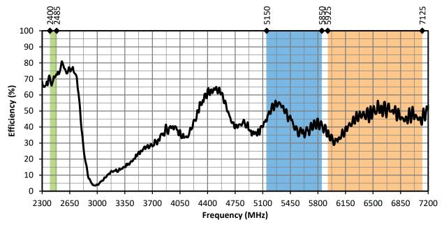
Figure 15. W63WS1 Antenna Radiation Efficiency, Edge-Bent
