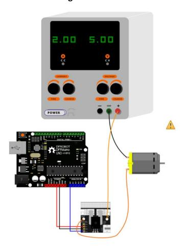
**DANGER:** This diagram can also be applied to AC current connection. But notice that the module should be cascaded on one electric wire (+/-). But if you connect it to two electric wires in parallel, you will short the circuit, which is dangerous.
