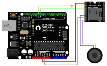
Note: For simple use , the upper diagram is ready, But if you find the noise is quite loud, then you could attach an 1K resistor to the TX pin.
