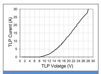
Fig.3 Transmission Line Pulsing (TLP) Measurement
