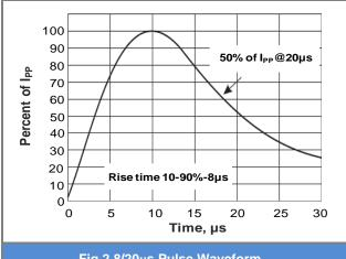
Fig.2 8/20µs Pulse Waveform
