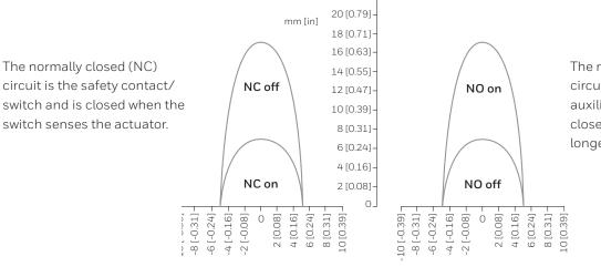
The normally open (NO) circuit is an optional auxiliary contact which closes when the switch no longer senses the actuator.
