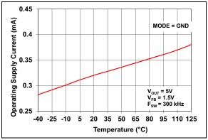
**FIGURE 2-16:** V<sub>IN</sub> Operating Supply Current vs. Temperature (MODE = GND).
