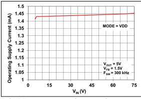
**FIGURE 2-13:** V<sub>IN</sub> Operating Supply Current vs. Input Voltage (MODE = VDD).
