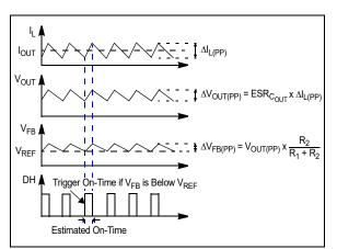
FIGURE 4-1: MIC28515 Control Loop Timing (CCM Mode).
