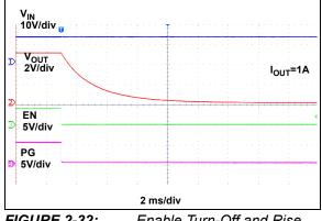
FIGURE 2-32: Enable Turn-Off and Rise Time.
