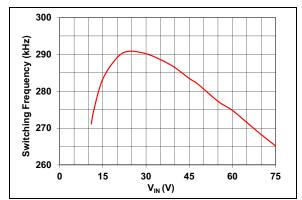
FIGURE 2-23: Switching Frequency vs. Input Voltage.
