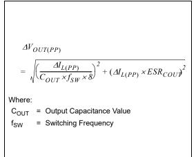
As described in Section 4.1 "Theory of Operation", a subsection of Section 4.0 "Functional Description", the MIC28515 requires at least 20 mV peak-to-peak ripple at the FB pin to make the  $g_m$  amplifier and the error comparator behave properly. Also, the output voltage ripple should be in phase with the inductor
