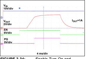
FIGURE 2-34: Enable Turn-On and Turn-Off.
