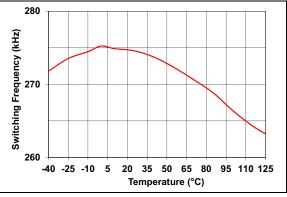
FIGURE 2-24:Switching Frequency vs.Temperature.
