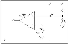
FIGURE 5-1: Voltage Divider Configuration.
