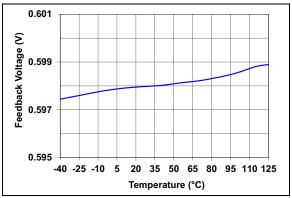
FIGURE 2-30:Feedback Voltage vs.Temperature.
