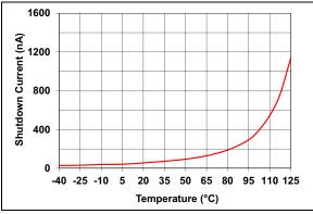
*FIGURE 2-18:* V<sub>IN</sub> Shutdown Current vs. Temperature.
