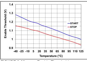
**FIGURE 2-22:** Enable Threshold vs. Temperature.
