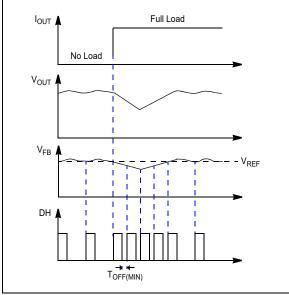
FIGURE 4-2: MIC28515 Load Transient Response.
