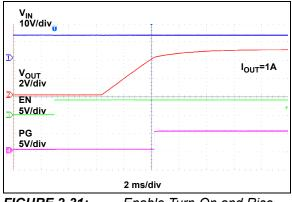
FIGURE 2-31: Enable Turn-On and Rise Time.
