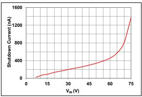
*FIGURE 2-17:* V<sub>IN</sub> Shutdown Current vs. Input Voltage.
