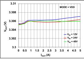
**FIGURE 2-7:** Output Voltage vs. Output Current ( $V_{OUT} = 3.3V$ ).
