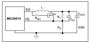
FIGURE 5-4: Invisible Ripple at FB.
