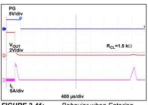
FIGURE 2-41: Behavior when Entering Short-Circuit.
