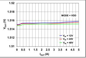
**FIGURE 2-5:** Output Voltage vs. Output Current ( $V_{OUT} = 1.5V$ ).
