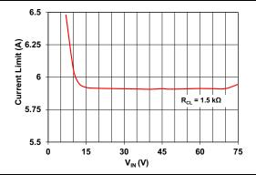
FIGURE 2-26: Output Current Limit vs. Input Voltage.
