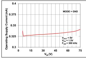
**FIGURE 2-15:** V<sub>IN</sub> Operating Supply Current vs. Input Voltage (MODE = GND).
