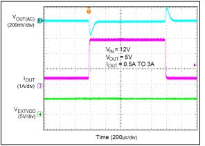
**FIGURE 4-4:** V<sub>OUT</sub> Load Transient with EXTVDD Connected to V<sub>OUT</sub>.
