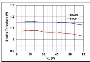
FIGURE 2-21: Enable Threshold vs. Input Voltage.
