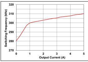
*FIGURE 2-25:* Switching Frequency vs. Output Current.
