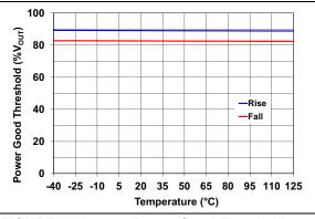
*FIGURE 2-28:* Power Good Threshold vs. Temperature.
