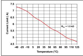
FIGURE 2-27: Output Current Limit vs. Temperature.
