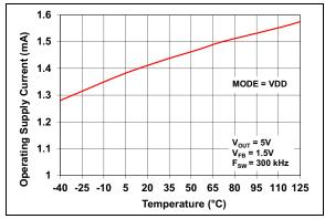
**FIGURE 2-14:** V<sub>IN</sub> Operating Supply Current vs. Temperature (MODE = VDD).
