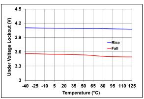
FIGURE 2-29: Undervoltage Lockout vs. Temperature.
