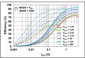
**FIGURE 2-4:** Efficiency vs. Output Current ( $V_{IN}$  = 48V).
