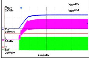
FIGURE 2-44: Recovery from Thermal Shutdown.
