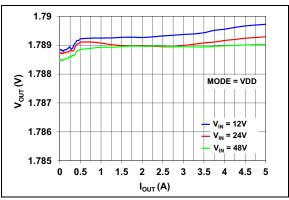
**FIGURE 2-6:** Output Voltage vs. Output Current ( $V_{OUT} = 1.8V$ ).
