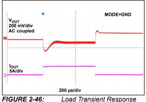
FIGURE 2-46: Load Transient Response (0 to 5A) - HLL.
