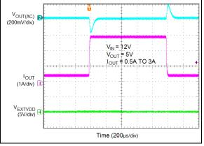
**FIGURE 4-5:** V<sub>OUT</sub> Load Transient with EXTVDD Connected to Ground.
