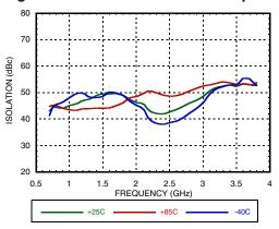
Figure 10. LO Leakage vs. Frequency<sup>[2][3]</sup>
