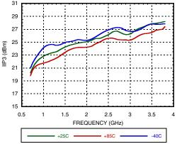
Figure 28. High Side LO Input IP3 vs. Frequency at VGATE=4.9V<sup>[2]</sup>
