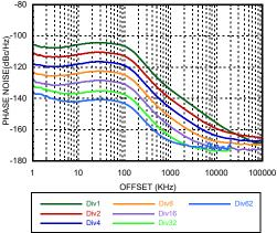
Figure 51. Auxiliary LO Output, Open Loop Phase Noise at 4100 MHz
