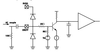
Figure 70. Reference Path Input Stage
