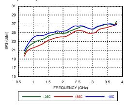
Figure 34. High Side LO Input IP3 vs. Frequency at VGATE=4.8V<sup>[2]</sup>
