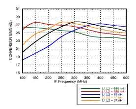
Figure 76. Conversion gain, IIP3 vs IF Frequency over IF Amplifier Choke Inductors [1][2]
