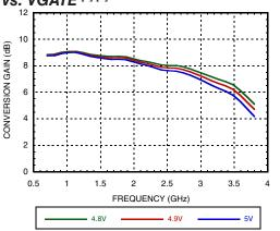
Figure 3. High Side LO Conversion Gain vs. VGATF [1] [2]
