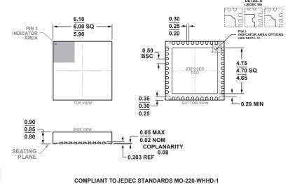
40-Lead Lead Frame Chip Scale Package [LFCSP] 6 mm × 6 mm Body and 0.85 mm Package Height (CP-40-19) Dimensions in millimeters
