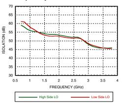
Figure 38. Channel to Channel Isolation vs. IF Frequency
