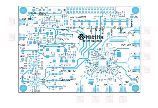
The circuit board used in the application should use RF circuit design techniques. Signal lines should have 50 Ohm impedance while the package ground leads and exposed paddle should be connected directly to the ground plane similar to that shown. A sufficient number of via holes should be used to connect the top and bottom ground planes. All evaluation board related drawings are available under Evaluation Kits tab of product page www.analog.com/HMC1190A
