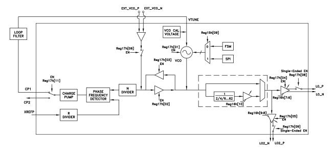
Figure 66. HMC1190ALP6NE PLL VCO Block Diagram
