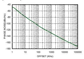
Figure 50. Auxiliary LO Output, Fractional Mode Closed Loop Phase Noise at 3600 MHz with various divider ratios [1]
