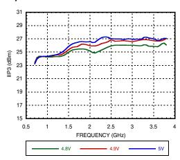
Figure 74. Conversion Gain & IIP3 vs. RF Frequency over VGATE Pin Voltage at 25C, IF =150 MHz
