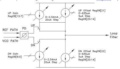
Figure 69. Charge Pump Gain & Offset Control
