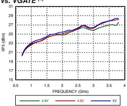
Figure 4. High Side LO Input IP3 vs. VGATE [1]
