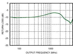
Figure 67. Auxiliary LO Single Ended Output Return Loss
