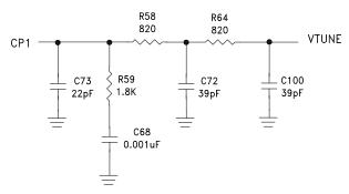
Figure 78. Loop filter components for HMC1190ALP6NE is configured as PLL alone used with external VCO HMC384LP4E
