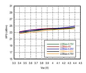
Figure 75. Conversion Gain, IIP3 vs. VCS1, VCS2 and LOBIAS2 voltages at 1900 MHz RF Input.
