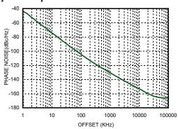
Figure 52. Auxiliary LO Output, Fractional Mode Closed Loop Phase Noise at 4100 MHz with various divider ratios [1]
