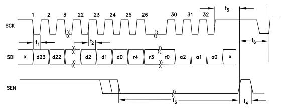
Figure 72. Serial Port Timing Diagram - WRITE
