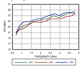
Figure 22. High Side LO Input IP3 vs. Frequency at VGATE=5V<sup>[2]</sup>
