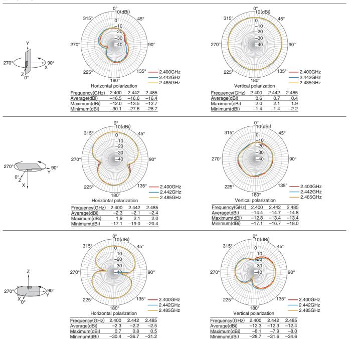
Tested antenna has been soldered. Evaluation board size is 50x20x1 mm.
