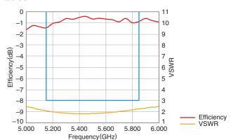
$\bullet$  Tested antenna has been soldered. Evaluation board size is 50x20x1 mm.
