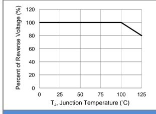
**Fig.5 Operating Temperature Derating Curve**
