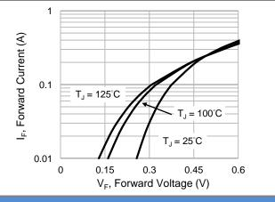
Fig.4 Typical Forward Characteristics
