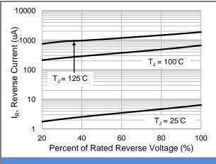
Fig.3 Typical Reverse Characteristics
