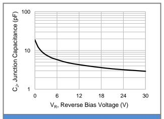
**Fig.2 Typical Junction Capacitance**
