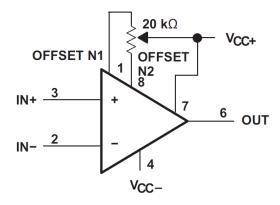
Fig 1. Input Offset Voltage Null Circuit
