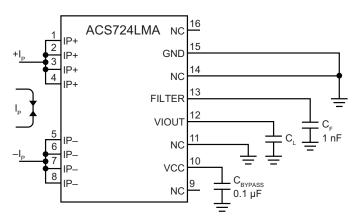
The ACS724LMA outputs an analog signal,  $V_{\rm IOUT}$ , that changes proportionally with the bidirectional AC or DC primary sensed current,  $I_{\rm P}$ , within the specified measurement range.
