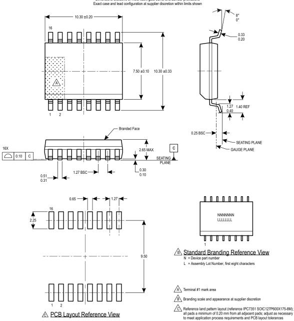
Figure 7: Package MA, 16-Pin SOICW
