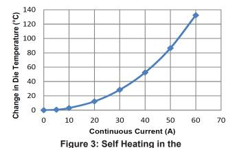
MA Package Due to Current Flow 80 70 Continuous Current (A) 60 50 40 30 20 10 0 175 25 50 75 100 125 150 Ambient Temperature (°C)
