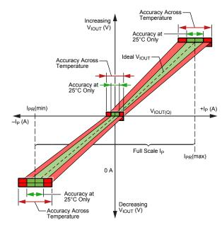
Figure 1: Output Voltage versus Sensed Current
