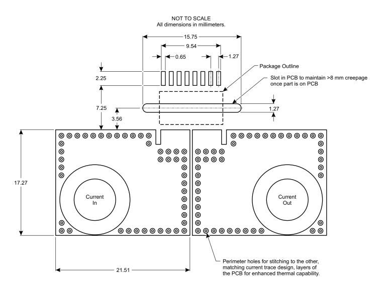
Figure 6: High-Isolation PCB Layout
