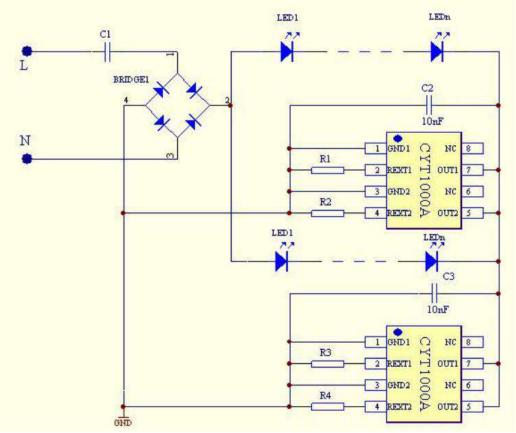
IC control LEDs in Parallel respectively
