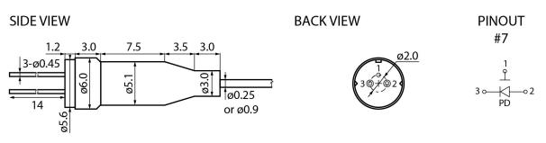
Connector FC/UPC, FC/APC, no connector, or by request
