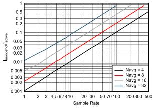
Figure 10. Illumination Supply Current in Monoshot Mode
