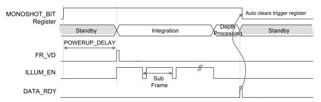
Figure 16. Timing for Register (MONOSHOT\_BIT) Triggered Monoshot Mode
