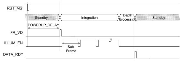
Figure 15. Timing for Pin-Triggered Monoshot Mode With RST MS
