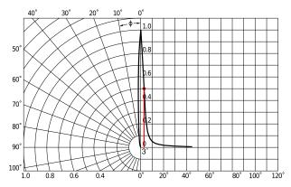
Figure 170. SFH4550 LED Radiation Characteristics
