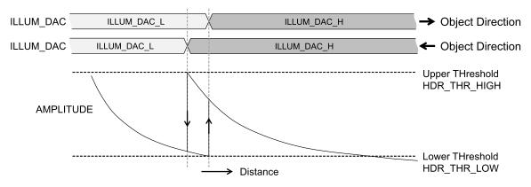
Figure 20. HDR Mode Operation With Distance
