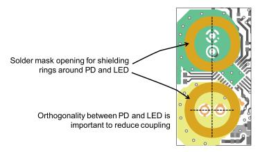
Figure 181. Photodiode and LED Placement on PCB
