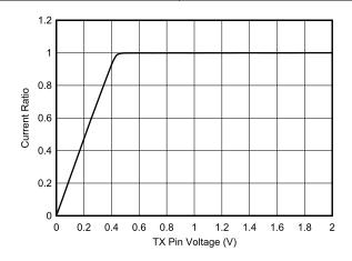
Figure 3. Illumination Driver I-V Characteristics
