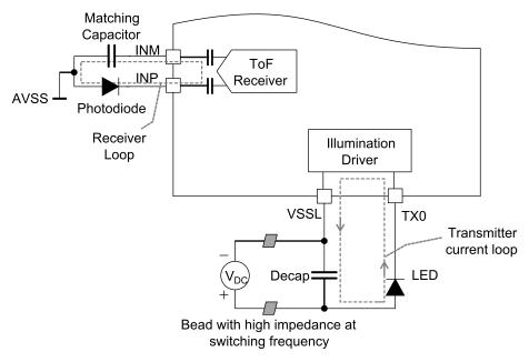
Figure 178. AFE Interface With Photodiode and LED
