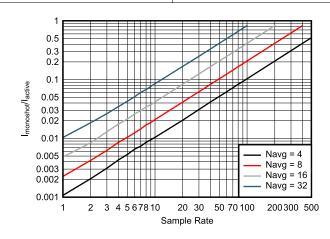
Figure 13. Illumination Supply Current in Monoshot Mode With Internal LDO
