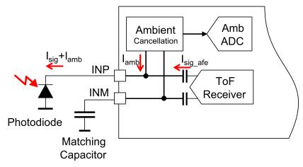
Figure 21. AFE, Photodiode Interface
