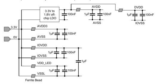
Figure 176. Power Supply Network in a System With External 1.8-V Regulator
