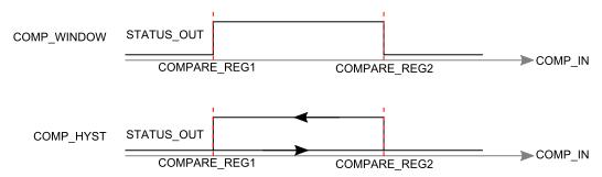
Figure 24. Interrupt Output Using Different Comparison Commands
