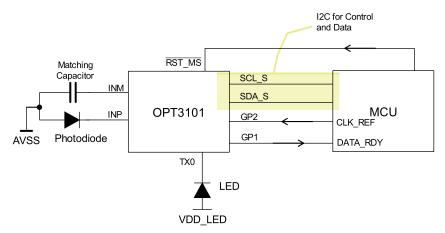
Figure 169. Typical Application Block Diagram
