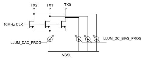
Figure 23. Illumination Driver Block Diagram
