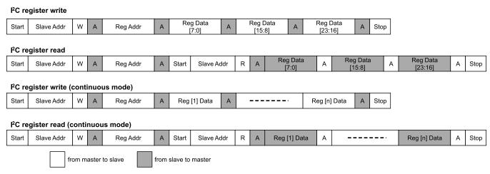
Figure 27. I<sup>2</sup>C Slave Interface R/W Modes
