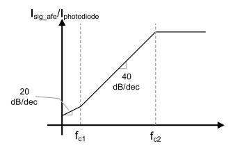
Figure 22. Ambient Cancellation Circuit Frequency Response
