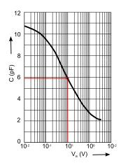
Figure 172. SFH213FA Photodiode Reverse Bias Capacitance
