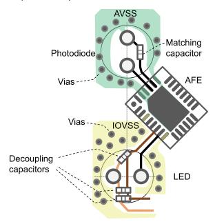
Figure 179. PCB Layout example
