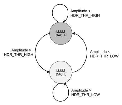
Figure 18. Auto HDR Mode: State Diagram
