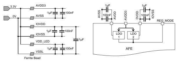
Figure 177. Power Supply Network With On-Chip 1.8-V Regulator
