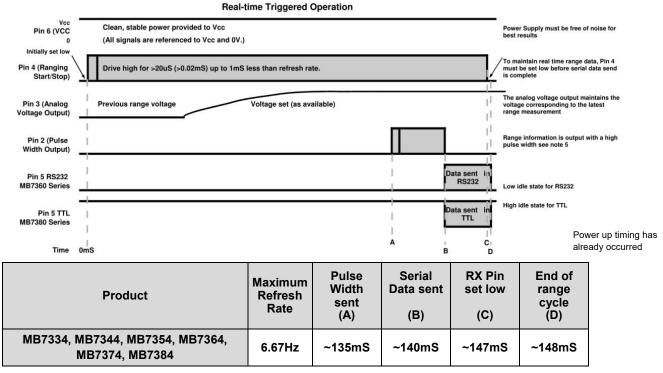
Real-time or triggered operation allows users to take advantage of a few functions unavailable during free run mode. When operating in triggered mode, an unfiltered maximum refresh rate can be achieved. This triggered operation allows users to range targets moving away from or closer to the sensor faster than 240mm per reading.
