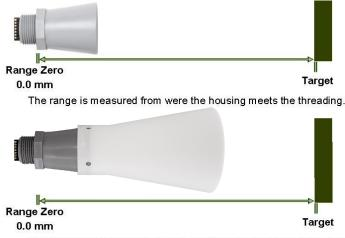
The range is measured from were the housing meets the threading.
