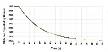
MB7354 responding to a 4 centimeter change. This shows the 7-mm rate limit along with the exponential filter.
