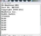
The serial data format is 9600 baud, 8 data bits, no parity, with one stop bit (9600-8-N-1). On power up the sensor will send serial data about the sensor. <u>View an example here</u>.
