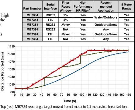
Nop (red): MB7364 reporting a target moved from 1 meter to 1.1 meters in a linear fashion. Middle (green): MB7334 responding to the same target, notice the steps when the target moves > 2%.
