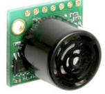
The LV-ProxSonar-EZ allows users to integrate several sensors into one system and experience little to no effect from the sensor interference than can occur with other ultrasonic sensor solutions. The LV-ProxSonar-EZ features an easy to use logic level (high/low) output, and RS232 format serial output. \*Factory calibration and testing is standard.
