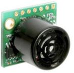
incredibly small package. The ParkSonar-EZ sensor allows users to integrate several sensors into one system and experience little to no effect from the sensor interference than can occur with other ultrasonic sensor solutions. ParkSonar-EZ sensor features an easy to use logic level (high/low) output, and RS232 format serial output. \*Factory calibration and testing is standard.
