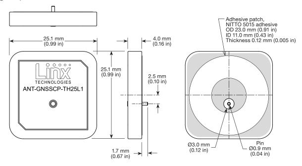
Figure 1. GNSSCP-TH25L1 Antenna Dimensions
