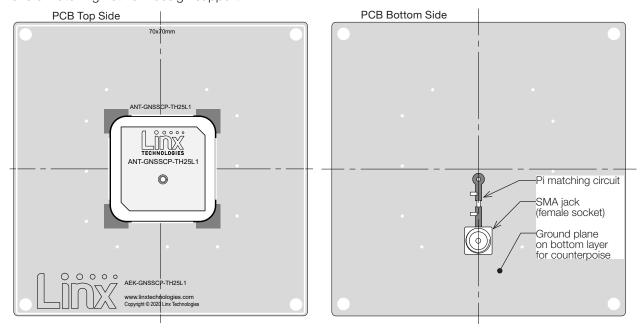
Figure 9. Recommended PCB Layout for the GNSSCP-TH25L1
