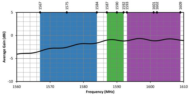
Figure 5. GNSSCP-TH25L1 Antenna Average Gain
