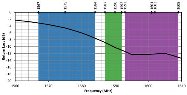
Figure 3. GNSSCP-TH25L1 Return Loss
