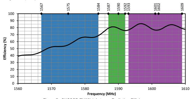
Figure 7. GNSSCP-TH25L1 Antenna Radiation Efficiency
