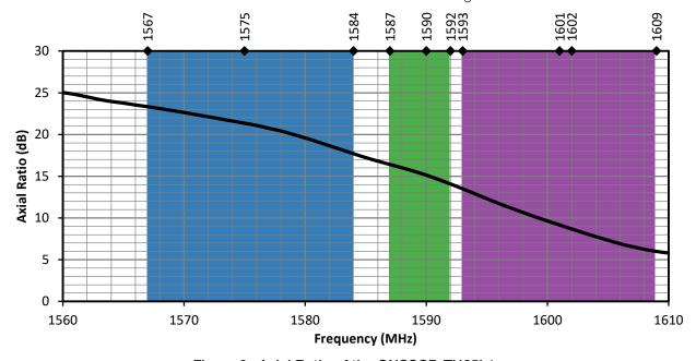
Figure 6. Axial Ratio of the GNSSCP-TH25L1
