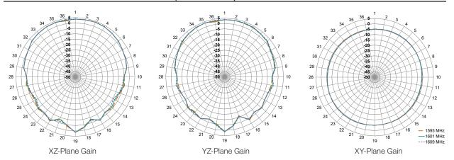
Figure 8. ANT-GNSSCP-TH25L1 Radiation Patterns
