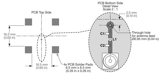
Figure 11. ANT-GNSSCP-TH25L1 Antenna Placement on PCB
