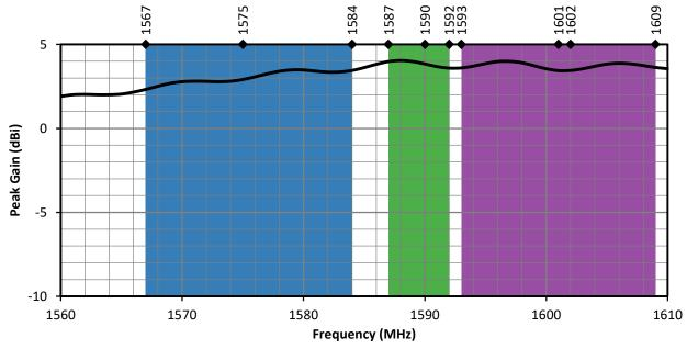
Figure 4. GNSSCP-TH25L1 Peak Gain
