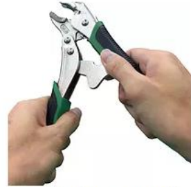
Quick release: Just pull the handles with both hands
