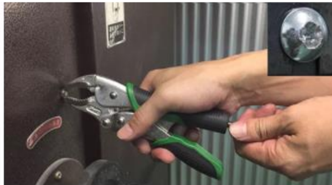
Step 2 : Adjust the opening jaws with the bolt to fit the diameter of a screw.
