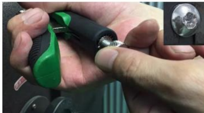
Step 3 : Fasten the adjusting bolt further (half a turn to the right)
