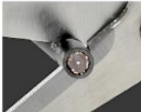
Coaxial cable (Conductor dia. 1.0mm)
