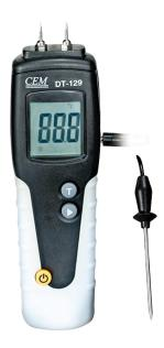
Conductivity moisture instrument designed for use in wood, used to measure the moisture level in sawn timber (also cardboard, paper) and hardened materials (plaster, concrete and mortar). They display the moisture level. The instruments have an average adjustment for European wood based on a wood temperature of 20°C.
