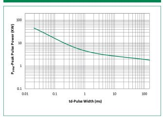
Figure 2 - Peak Pulse Power Derating Curve
