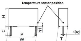
Note: If re-working or dipping twice is necessary, it should be done after the capacitor returns to the normal temperature.
