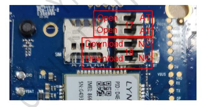
Figure 2-7 Serial port switch
