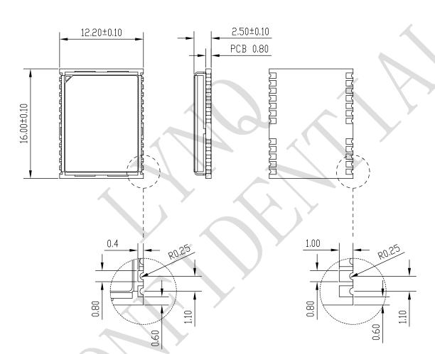
Figure 3 N20 mechanical dimensions (Unit: mm)
