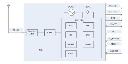
Figure 1 N20 functional diagram
