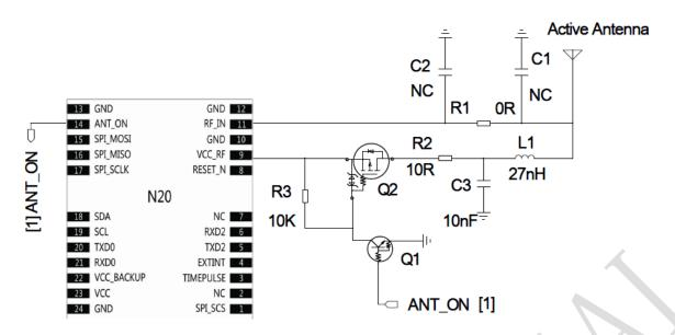
Figure 8 N20 Active antenna power consumption saving design
