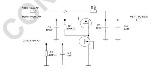
Figure3-5: PMOS (Reference circuit)
