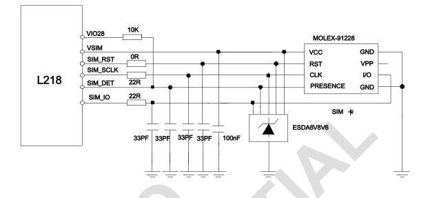
Figure 3-25: 8-pin SIM card(Reference circuit)
