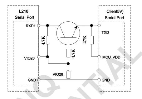
Figure3-23: 5VRXD level matching (Reference circuit)
