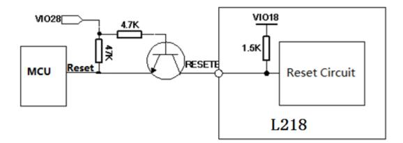
Figure3-10: Recommend the reset circuit: Key reset and MCU reset L218 Module
