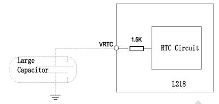
Figure3-13: External capacitor to the RTC power supply
