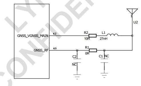
Figure 3-33:GNSS active antenna (Reference circuit)
