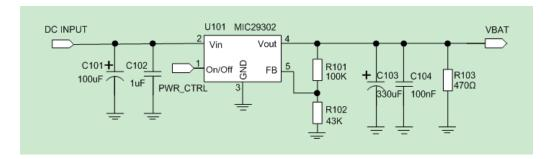
Figure3-3: LDO(Reference circuit)
