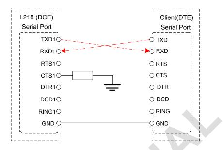
Figure 3-19: Serial port three line connection
