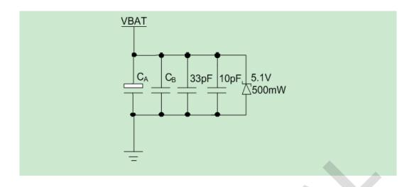
Figure3-2: VBAT input (Reference circuit)
