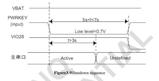
Note: As logout network time is related to the local mobile network, it is recommended to delay about 12 seconds before disconnecting the power supply or restarting the module.
