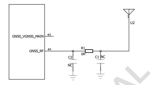
Figure 3-32:GNSS passive antenna (Reference circuit)
