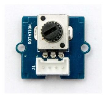
The rotary angle sensor produces analog output between 0 and Vcc (5V DC with Seeeduino) on its D1 connector. The D2 connector is not used. The angular range is 300 degrees with a linear change in value. The resistance value is 10k ohms, perfect for Arduino use. This may also be known as a "potentiometer".
