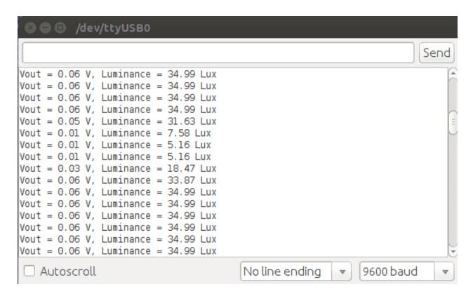
6. The Vout and Lux are displayed in the serial monitor.
