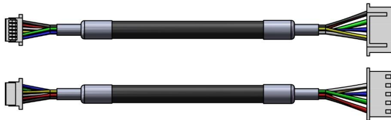
Figure 2-6 RPLIDAR S1 Interface Lead Schematic Diagram
