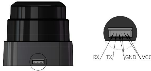
Figure 2-5 RPLIDAR S1 Female Receptacle Definition
