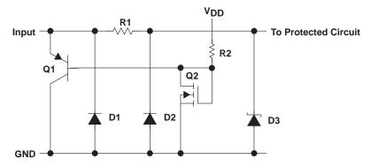
Figure 1. LinCMOS ESD-Protection Schematic
