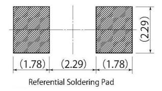
Optimize soldering pad to the board design and soldering condition.
