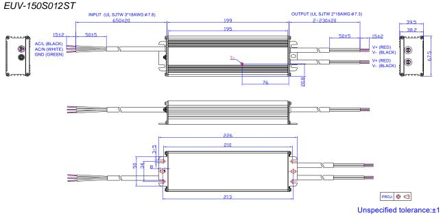
**Note:** The 2 DC output cables are connected in parallel internally because one AWG #18 wire can only carry 10A. Please connect the 2 red wires together and 2 black wires together in application, or ensure each cable carries same current.
