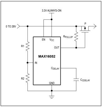
Figure 4. Overvoltage Protection
