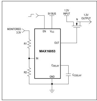
Figure 5. Low-Voltage Sequencing Using an nMOSFET
