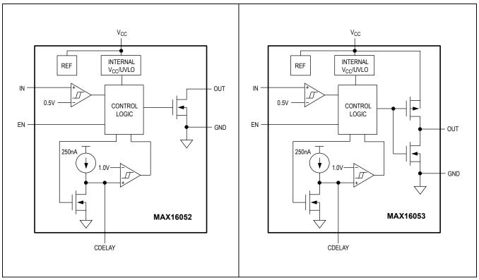
Figure 2. Simplified Functional Diagram
