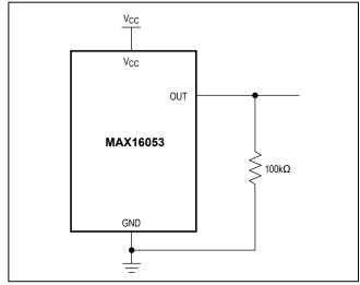
Figure 3. Ensuring OUT Valid to  $V_{CC} = 0V$
