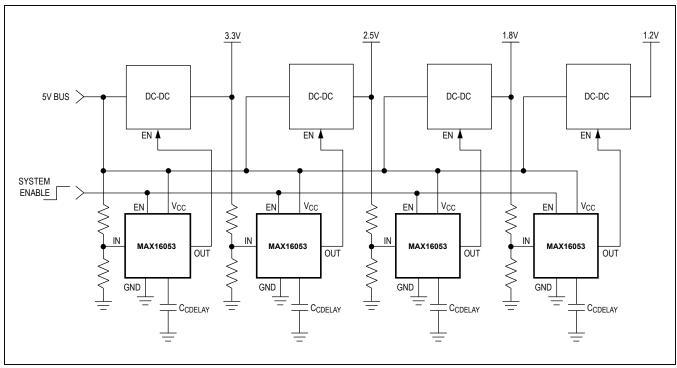
Figure 6. Multiple Output Sequencing
