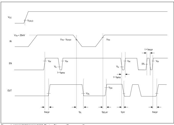
Figure 1. MAX16052/MAX16053 Timing Diagram (C<sub>CDELAY</sub> = 0)
