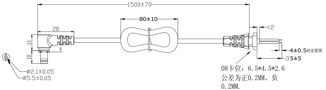
12.2 DC 输出线输出极性 (Polarity) : 见下图 as below
