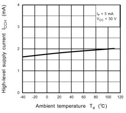
Fig. 13.2.6 I<sub>CCH</sub> - T<sub>a</sub>
