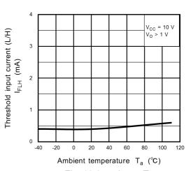
Fig. 13.2.4 I<sub>FLH</sub> - T<sub>a</sub>
