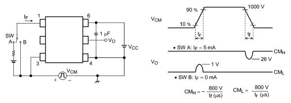
Fig. 13.1.8 Common-Mode Transient Immunity Test Circuit and Waveform
