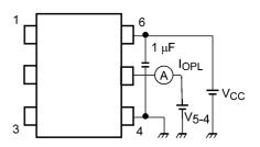
Fig. 13.1.2 I<sub>OPL</sub> Test Circuit
