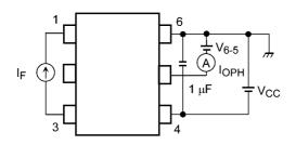
Fig. 13.1.1 I<sub>OPH</sub> Test Circuit
