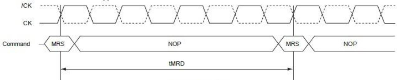
Figure 8  $t_{MRD}$  Timing
