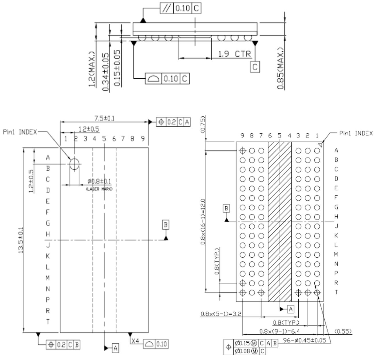
Figure 19 FBGA 96-ball package outline drawing (unit:mm)
