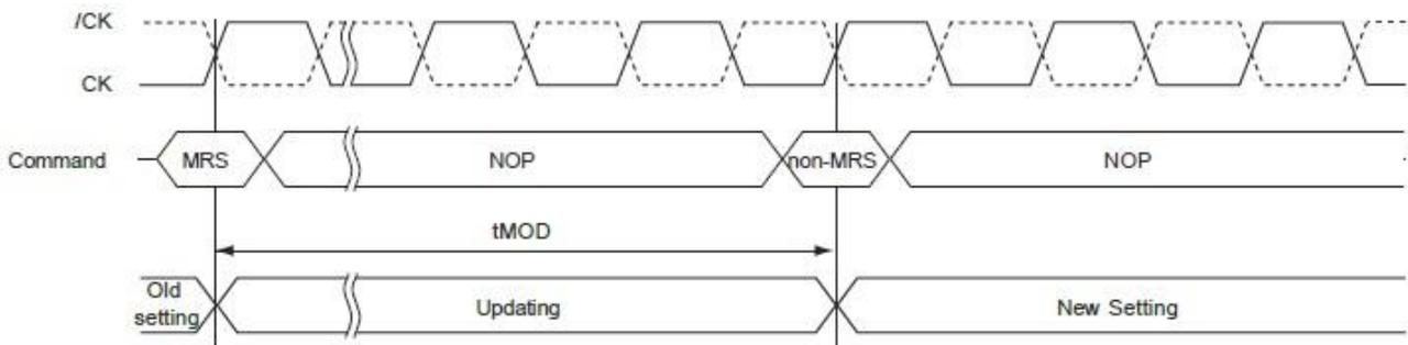
Figure 9  $t_{MOD}$  Timing
