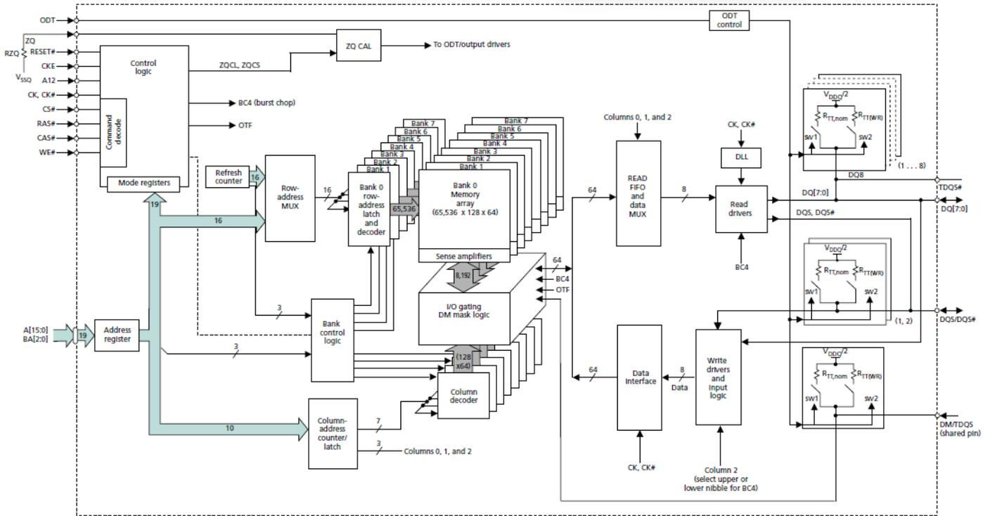
Figure 4 512Mx8 Functional Block Diagram
