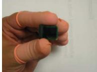
Fig. 3 Best method of handling the displays
