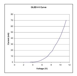
Figure 9-4. OLED I-V Characteristic (Log and Linear scale)
