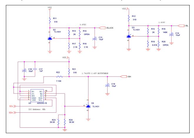
Figure 9-5. Sample Circuit Designs Using External References
