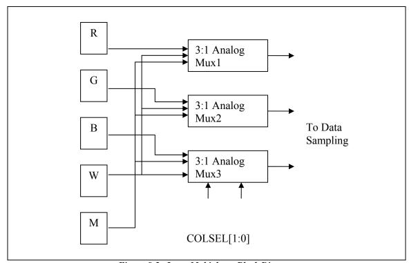
Figure-9-2. Input Multiplexer Block Diagram
