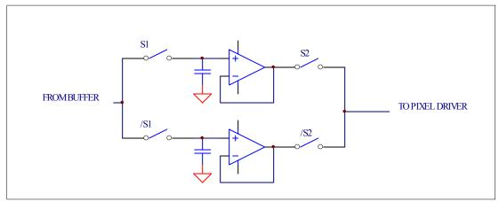
Figure 9-3. Dual Sample & Hold Block Diagram
