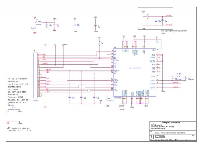
Figure 13-1. Microdisplay Carrier Board Electrical Diagram
