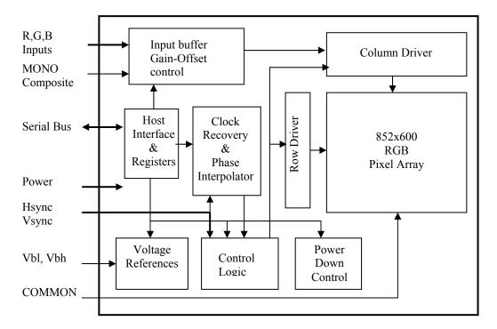
Figure 3-1. Microdisplay functional block diagram
