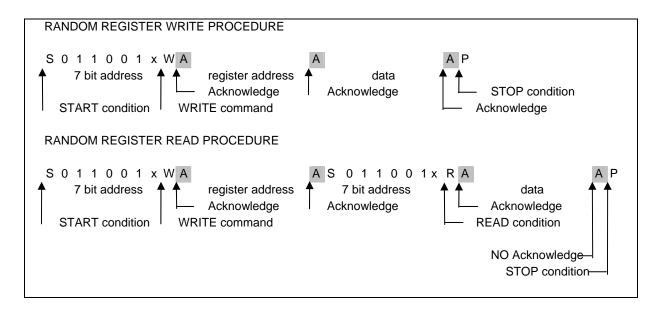
Figure 9-8. Serial Interface Protocol
