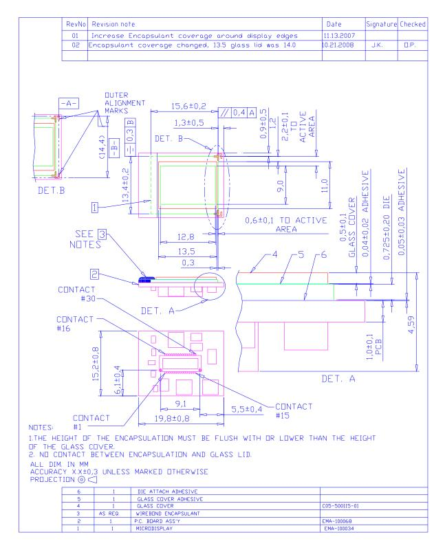
Figure 7-1. Mechanical Characteristics
