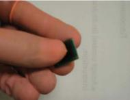
Fig. 4 Avoid this method of display handling
