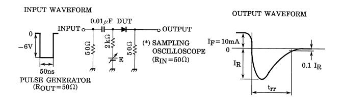
Fig.1 Reverse Recovery Time (trr) Test Circuit
