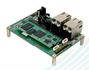
iWave's i.MX6UL development board incorporates i.MX6UL SODIMM SOM which is based on Freescale's power efficient i.MX6UL ARM Cortex A7 processor and the carrier board with optional 4.3" resistive display kit. The development board can be used for quick prototyping of various applications targeted by the i.MX6UL processor. With the 100mm x 72mm Pico ITX size, and the kit is highly packed with all the necessary on-board connectors to validate the i.MX6UL CPU features.
