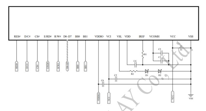
R2 = 50Ω, 1/8W D1, D2= 1N4148 C1, C2=4.7uF C3=0.1uF C4, C5, C6=1uF
